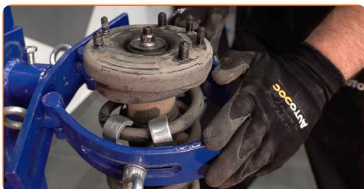
Remplacement : ressort de suspension – HONDA Accord VIII Break (CW).
